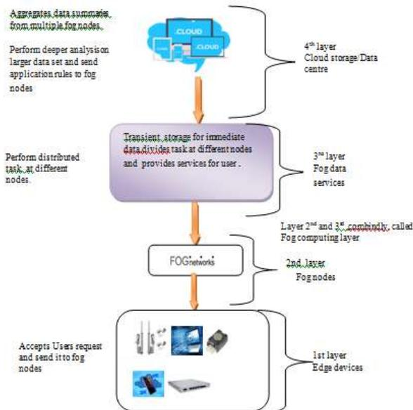
Figure 1.2: System Layered Architecture of Fog Computing
