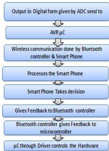
Fig c) Flowchart showing operation of AVR with smart phone.
