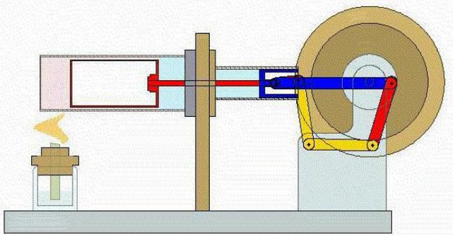
expanded in the hotter portion resulting in a net conversion of heat into work. An internal Regenerative heat exchanger increases the Stirling engine's thermal efficiency compared to simpler hot air engines lacking this feature.
