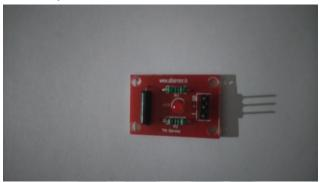
Figure 6. Mercury tilt sensor module
