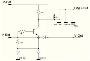
Figure 9. Supply Selector Switch
