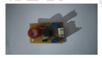
Figure 5. CO gas sensor module
