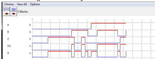
Fig 10: Timing Diagram of 12T Full adder
