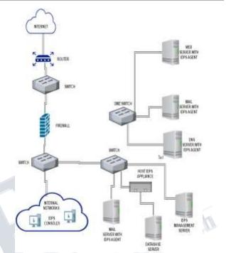
Fig1: Host Based IDPS Agent Deployment Architecture
