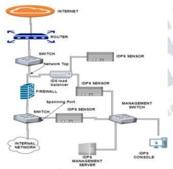
Fig3: Passive Network-Based IDPS Sensor Architecture
