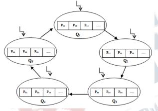
Elbow arrow in diagram shows that scheduler can pick first packet from any of queue for transmit initially. And arrow shows direction of scheduler after completion of each time quantum. Here 'Q' denotes queue while 'P' denotes packets of each respective queue. State transition probabilities for the above scheme will be
