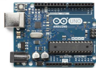
Fig. 2 Arduino UNO board. [11]
