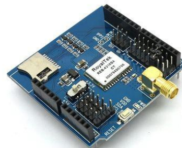
Fig. 3 Arduino GPS Shield. [12]
