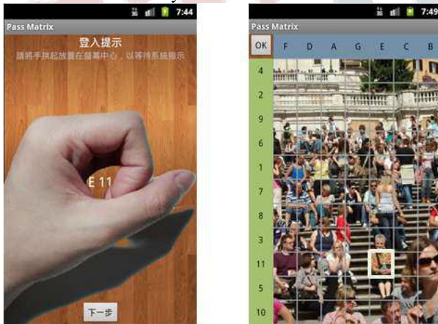
Fig. 7. (a) Obtain the login indicator (E,11) directly. (b) Obtain the login indicator through a predefined image.
