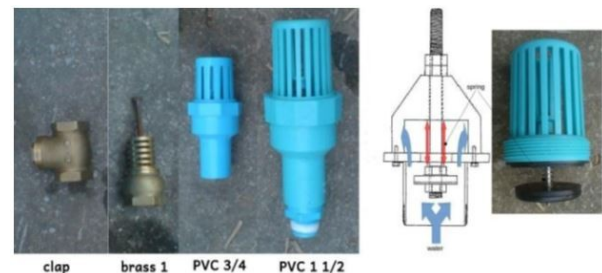
Figure 4. Different valves tested as impulse valve in the construction of a hydraulic ram, schematic view and disassembled manipulated inlet valve
