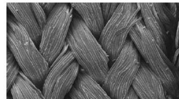
fig 4 A grayscale(microscopic) image of the silk fibre
