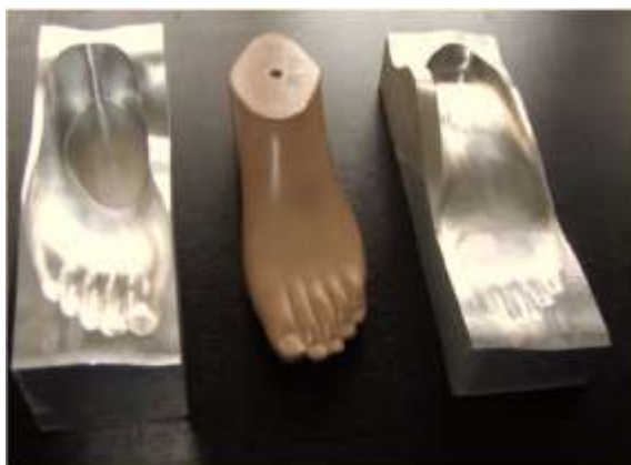
Figure 3: Injection molds and the original prosthetics in the middle.
