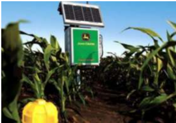
Figure 2: John Deere's Field Connect system used to collect soil, moisture and other data
