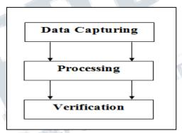
Common Block Diagram for working of all Biometric is:
