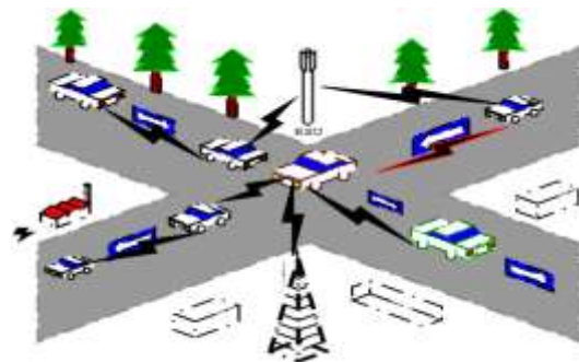
Figure 2: vehicular network architecture
