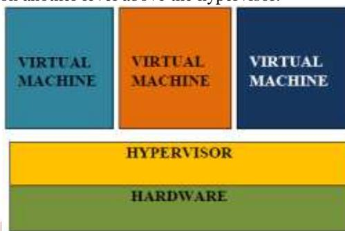
**Figure 3 Bare-Metal Virtualization**
