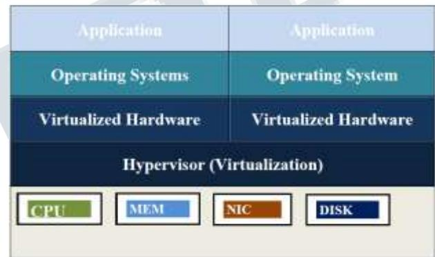
Figure 2 Virtualization Architecture
