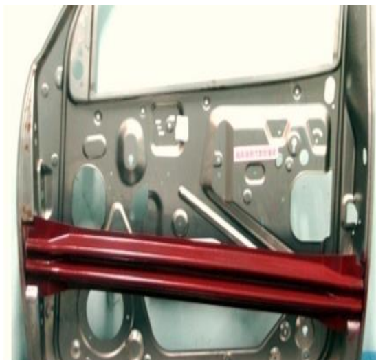
Figure 2: Ultra-high strength steel lightweight door beam
