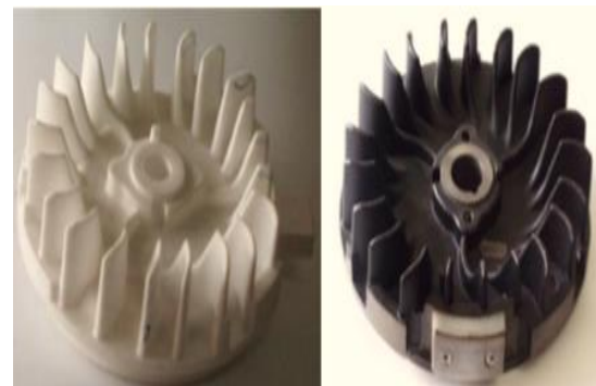
(a) Lost pattern (b) Casting part
