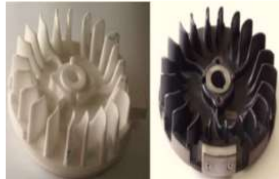
(a) Lost pattern (b) Casting part
