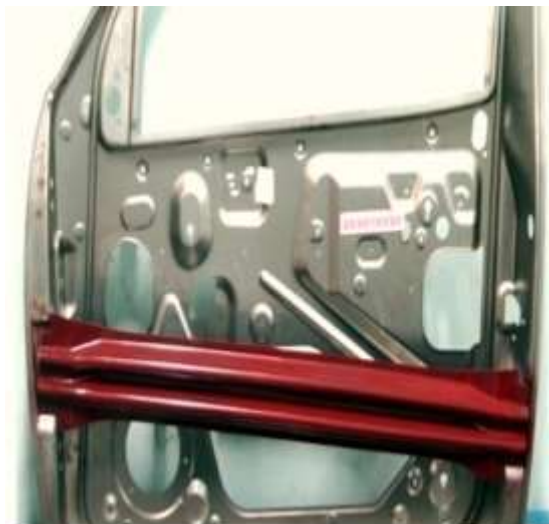
Figure 2: Ultra-high strength steel lightweight door beam
