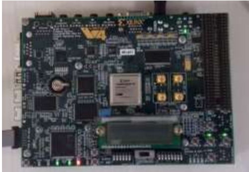
Fig. 9: A Virtex-4 ML401 FPGA Development Board.
