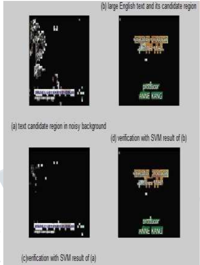
Fig. 3. (a) Text candidate region in noisy background; (b) Large English text ; (c) Verification with SVM results of (a) ; (d) Verification with SVM results of (b)
