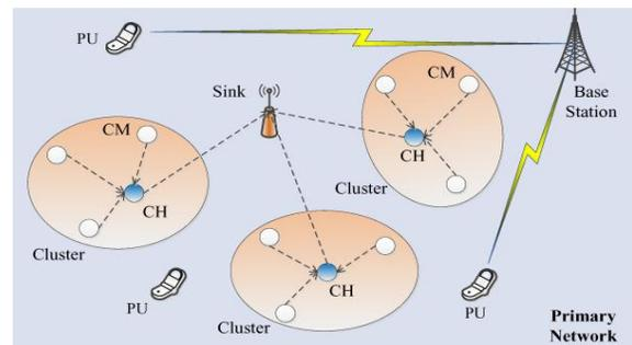
**Fig. The architecture of CRSN**
