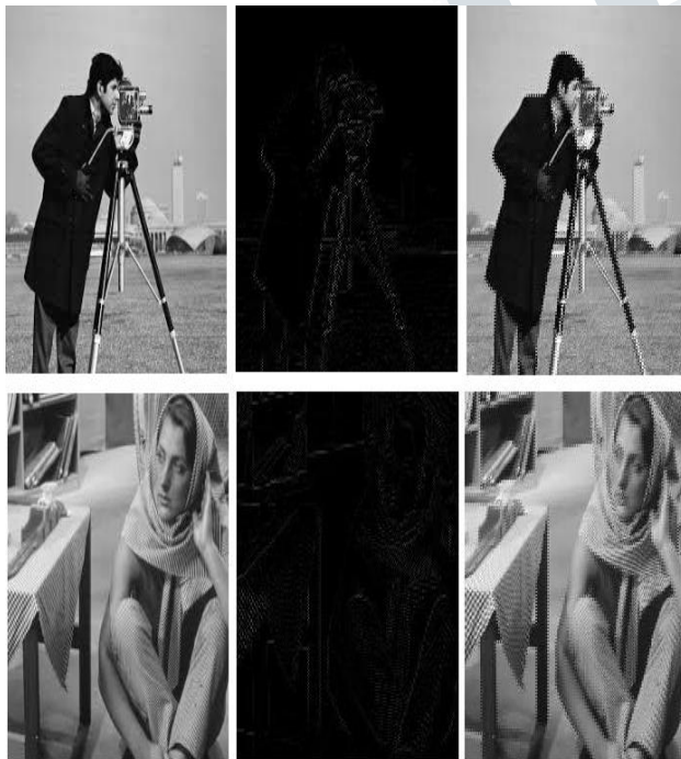
Figure 7. From top to bottom, standard test image Cameraman and Barbara, from right to left, the figure presents the Original, Encrypted and Decrypted algorithm results.
