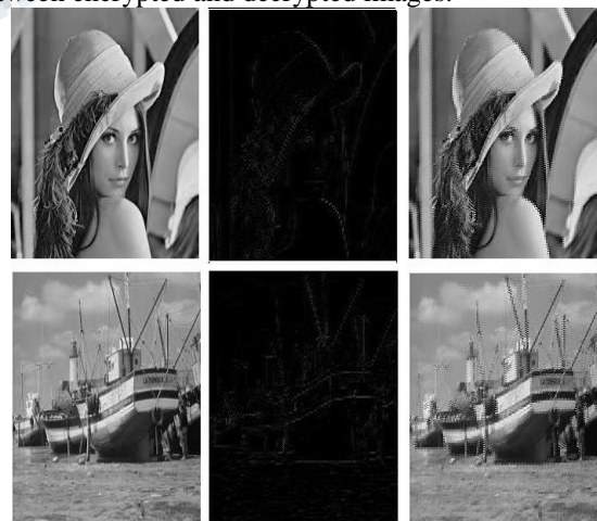
Figure 5. From top to bottom, standard test images Lena and Boat, from right to left, the figure presents the Original, Encrypted and Decrypted algorithm results.
