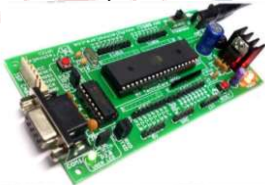
Fig. 1 8051 Development Board (AT89S52)
