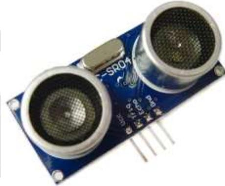
*Fig 5. Ultrasonic Sensor*
