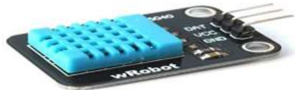
A humidity device (or hygrometer) insights, measures and aptitudes the comparative moistness in the midcourse. It accordingly measures in cooperation wetness and air temperature. Comparative humidity is the percentage of fixed moisture in the air to the highest quantity of dampness that can be interned at that air high temperature.
