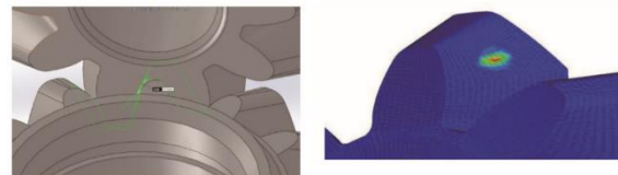
Figure 3: Backlash and Contact Tooth Position
