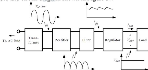
**Figure: Block diagram of power supply**
