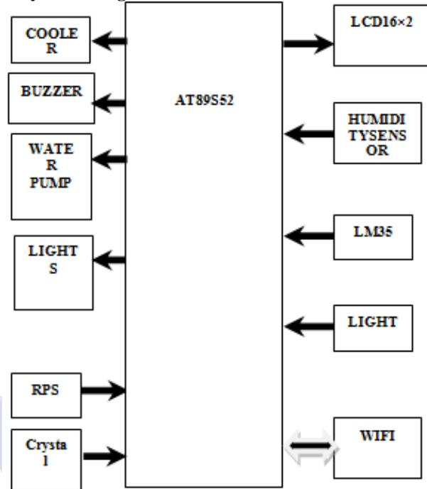
**Fig3.1: Block diagram of microcontroller**
