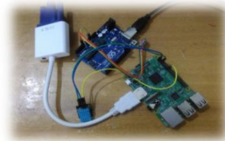
Fig. 7 Hardware of Mounting Temperature Sensor and Heartbeat Sensor
