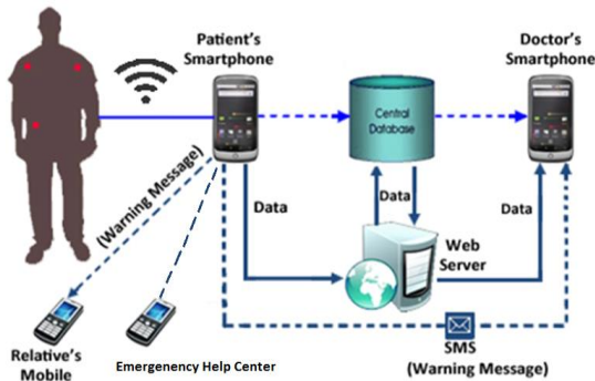
Fig.1 Logic Diagram of Patient Health Monitoring System [3]
