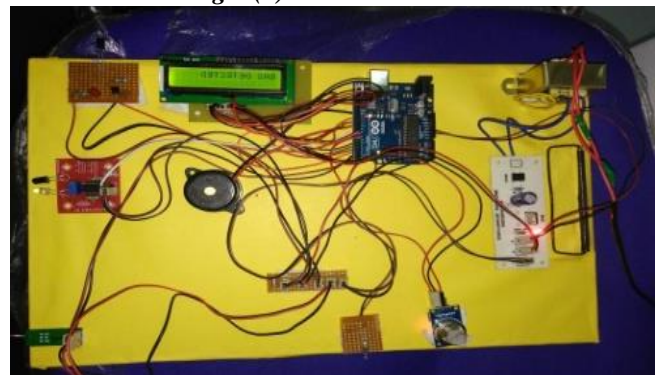
Fig. 4(b): Hazardous Gases are detected.
