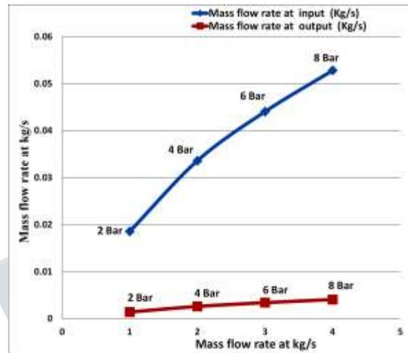
**Figure 47. Comparison plots for mass flow rate inside seal for the 13-degree angle between teeth seal profile**
