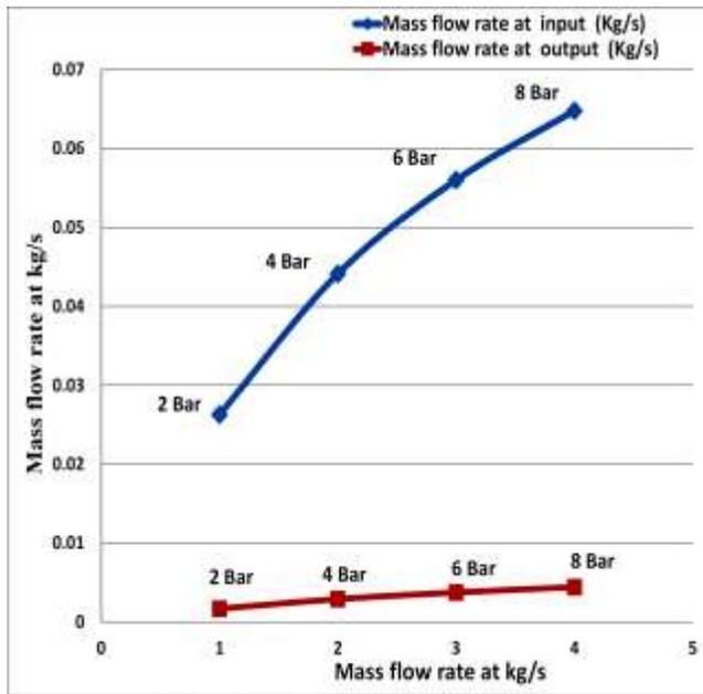
**Figure 46. Comparison plots for mass flow rate inside 0.5mm width of teeth seal profile.**
