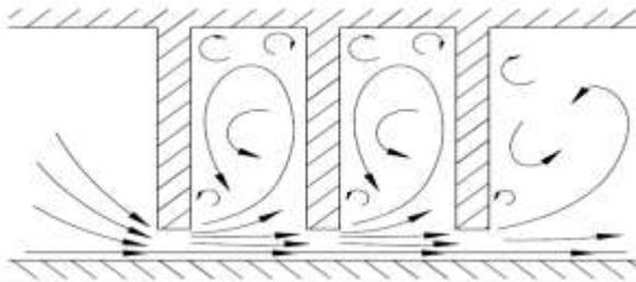
**Figure 2. Flow restriction in three Knives of the labyrinth seal**
