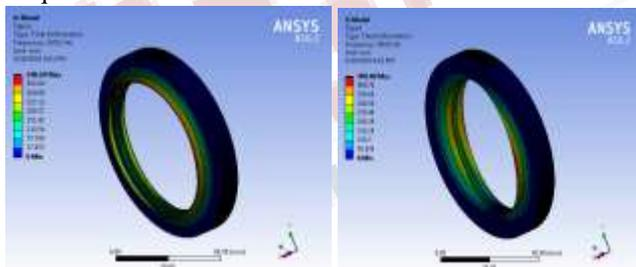
**Figure 9. & Figure 10. First and second mode shapes**
