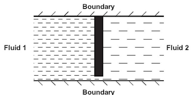
Figure: 1. Basic sealing geometry
