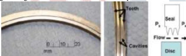
**Figure 3. Three knives labyrinth seal**
