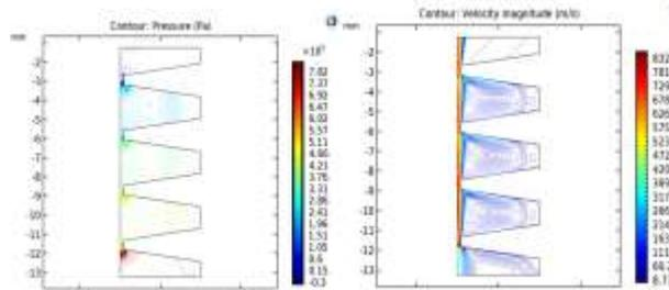
**Figure 20. & Figure 21. Pressure & Velocity contours for 8 bar inlet pressure**
