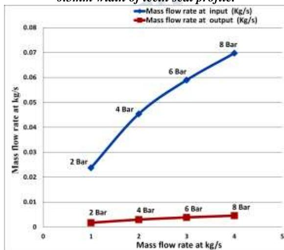
**Figure 45. & Comparison plots for mass flow rate inside 1mm width of teeth seal profile.**
