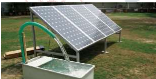
Figure:6 Solar water pump
