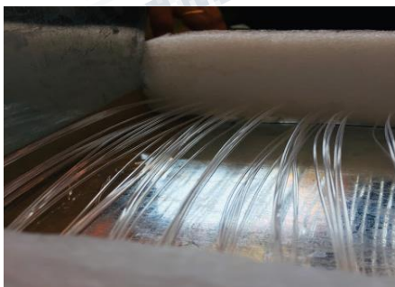
Fig 1 Inserting of optical fibers
