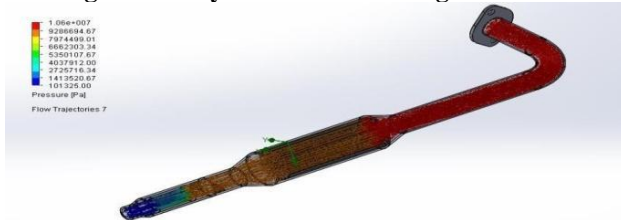
Fig.8 Pressure distribution through catalytic converter
