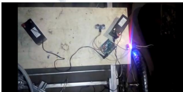
Fig.6.7 Test setup of Automatic Braking System
