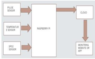
Fig. 1. Architecture of proposed system.
