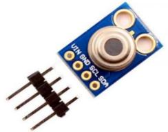
Fig. 2.3. Contactless Temperature Sensor
