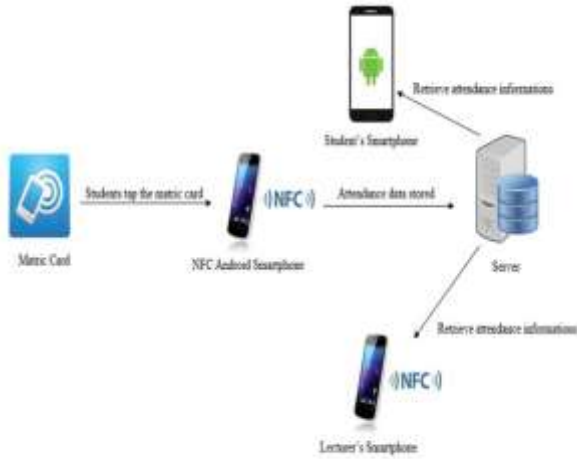
Fig 4: NFC Based Attendance System Architecture [13]
