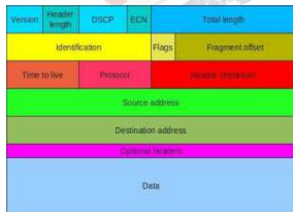
Fig. 2 IPv4 Header Frame Format
