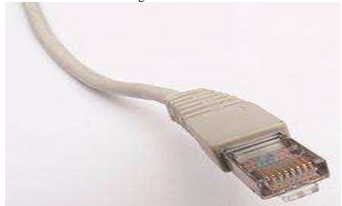
Fig. 5 Ethernet Local Area Network
