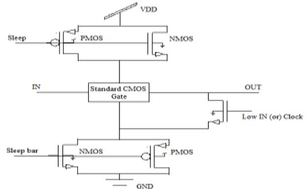
Fig. 4. DML Dual Sleep method (Type B topology)
