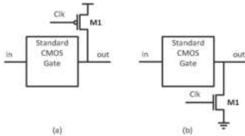
Fig. 1. Proposed basic DML gate. (a) Type A topology. (b) Type B topology.
