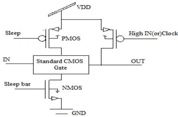
Fig. 3. DML Sleep method (Type A topology)
