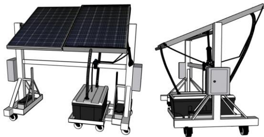
Figure 2. System mechanical design
