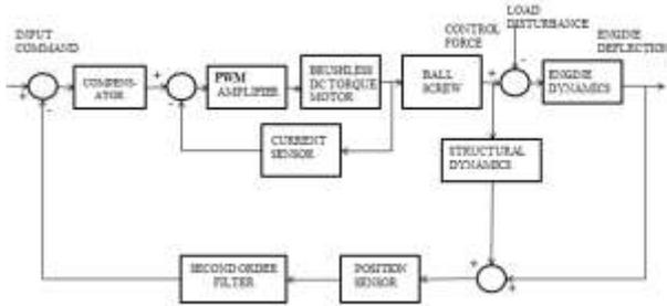
Fig.2. Block diagram of an actuator used in launch vehicle application
