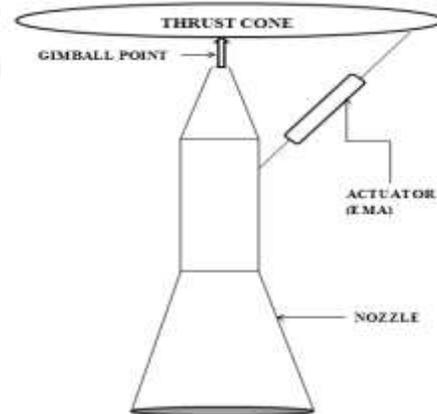
Fig.1. Schematic diagram of TVC servo actuation system
