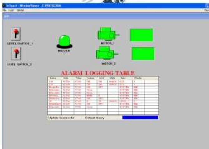
Fig.3 (b) snapshot of process monitoring in SCADA
