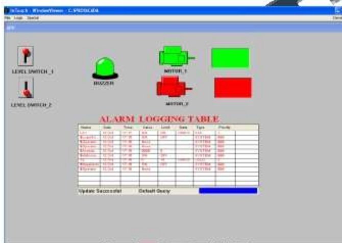
Fig.3 (a) snapshot of process monitoring in SCADA
