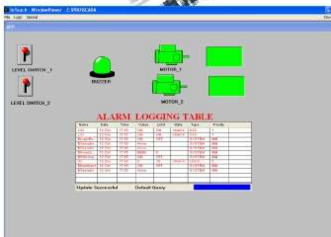
Fig.3 (b) snapshot of process monitoring in SCADA
