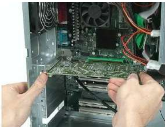
Fig.5a: PCI slots of CPU for interfacing with GPU
