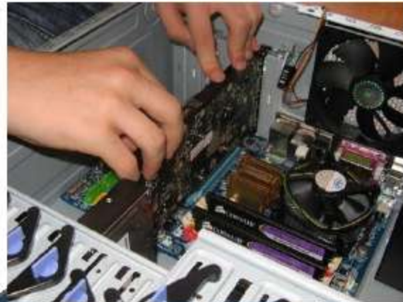
Fig.5b: Graphics card interfaced to PCI slot of motherboard
