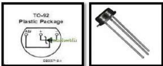
Fig. 9 connection digram of LM-236-5 reference diode
