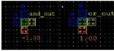
Figure 6. QCA layouts of AND gate and OR gate
