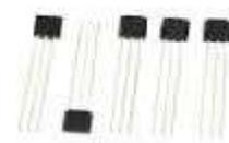
Fig.1 : hall effect sensor array
