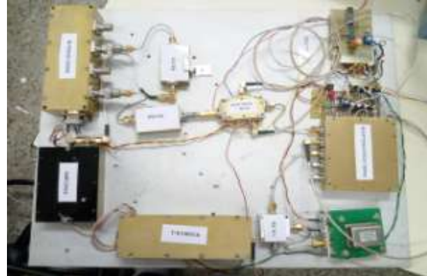
Fig: 15 Complete Signal Generator unit
