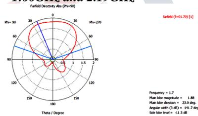
**Fig. 2. Directivity of the Proposed antenna at 1.7GHz**
