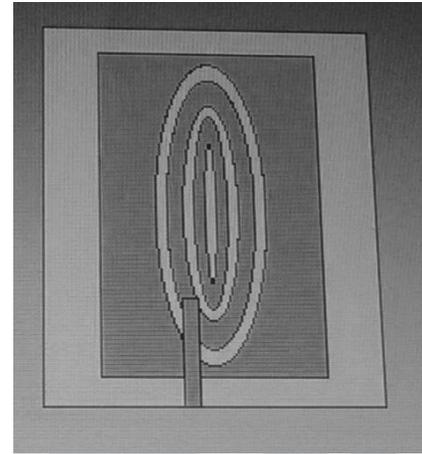
**Fig. 3. Proposed Elliptical Slotted MSPA**
