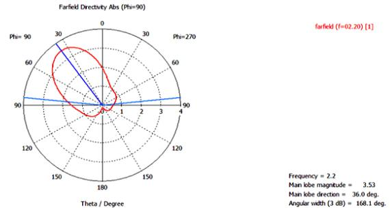
**Fig. 4. Directivity of the Proposed antenna at 2.2GHz**
