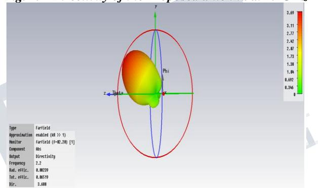
**Fig. 5. Directivity of the Proposed Antenna at 2.2GHz**
