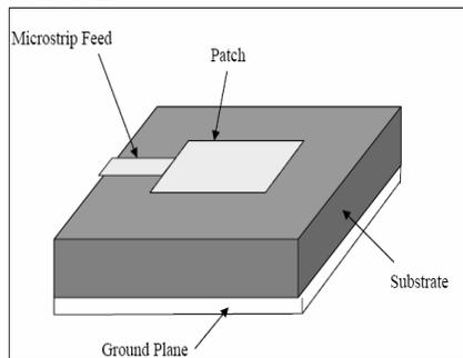
**Fig. 2. Microstrip patch antenna with Line Feed**
