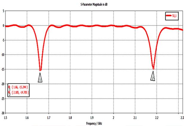
**Fig. 1. Return Loss of the Proposed antenna at 1.66GHz and 2.19GHz**
