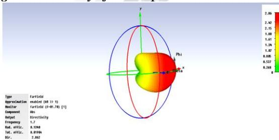
**Fig. 3. Directivity of the Proposed Antenna at 1.7GHz**
