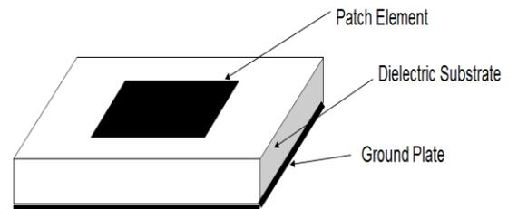
**Fig. 1. Basic Microstrip Patch Antenna**
