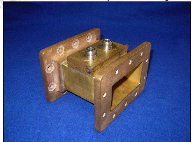
Fig.3. Fabricated 4-port dual directional coupler
